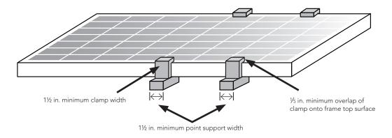
Figure 10: Point support and clamp requirements
